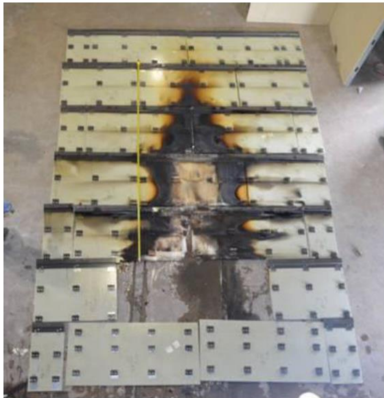
Figure C-17. Post Test Assembly Dissection – Interior Surface of StoneLite® Panels (SP-1-10-3) Panels following Exposure.
