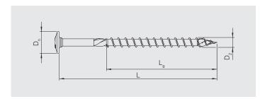
Flange head | T-drive | Partial or full thread Bright zinc plated, A3K | Carbon steel
