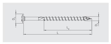
Flange head | T-drive | Partial thread 304 Stainless steel (A2 1.4567)
