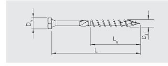
Combination hexagon head |T-drive Partial or full thread | Bright zinc plated, A3K | Carbon steel
