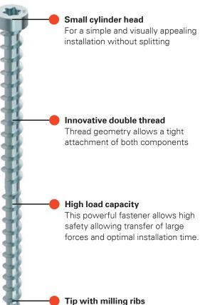
Noticeable reduction in the risk of wood-splitting together with fastener installation speed
