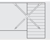
Cylinder head |T-drive | Double thread Bright zinc plated (A3K)
