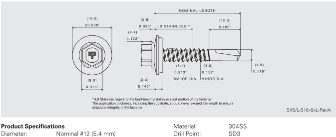
Diameter:Nominal #12 (5.4 mm)Threads Per Inch:11Head Style:5/16" dia HWH AFL (8.0 mm)Washer:5/8" stainless and EPDM bond seal<br/>(16 mm)
