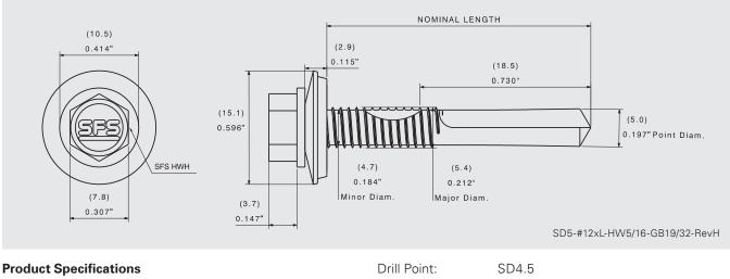
Diameter: #12 (5.4 mm) Threads Per Inch: 24 Head Style: 5/16" dia. HWH AF (7.8 mm) Washer: 19/32" galvanized and EPDM bond seal (15.1 mm)
