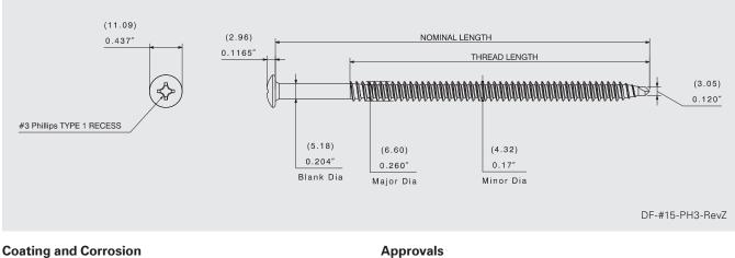
15/15 Kesternich per FM 4470 800 hour salt spray per ASTM B117 Cathodic epoxy e-coat
