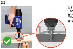
2.2 There can be a gap between the TU-fastener head and the bracket
