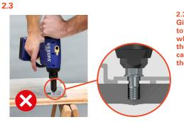
2.3 Giving heavy force to the TU-fastener while not removeing the mandrel can cause damage to the panel
